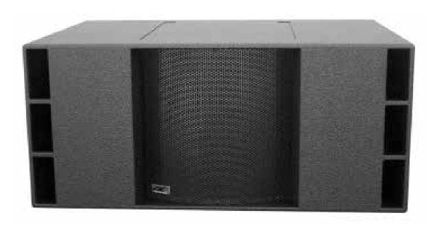
The Acoustic Technologies Groundswell 6000 is the latest generation low frequency cabinet. A fundamentally new design approach was applied early in the design stages utilising a complex combination of tuned reflex and partial short horn loading techniques. The result is a sub bass loudspeaker system of truly exceptional performance employing two 3000 Watt 18" transducers providing a full power response to 25Hz at anunrivalled sensitivity of 101dB at 1 watt, 1 metre.
