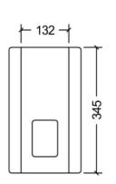
The Acoustic Technologies SS10 is an ultra-compact trapezoidal shaped cabinet constructed of premium Finnish Birch plywood and finished in extremely durable AcoustiCoate black elastomer with a black powder coated grille.
